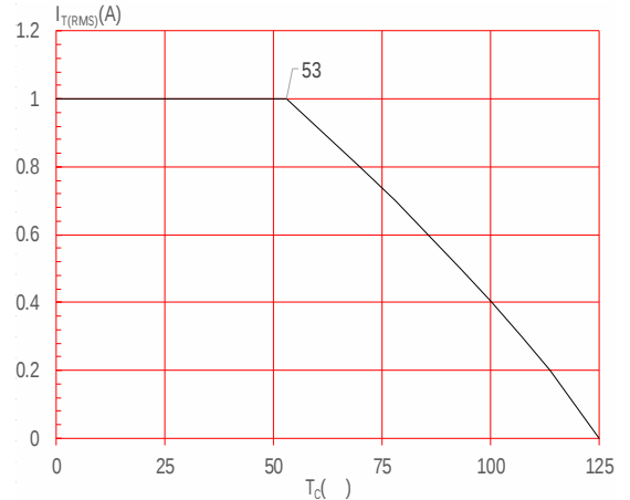
RMS on-state current versus case temperature
